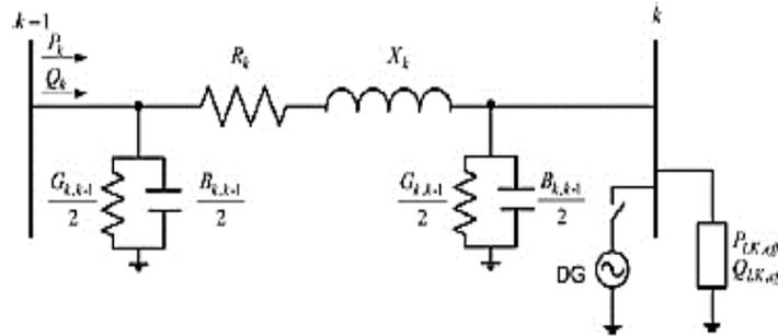
**Figure 2.** Simple Radial System with Feeder
