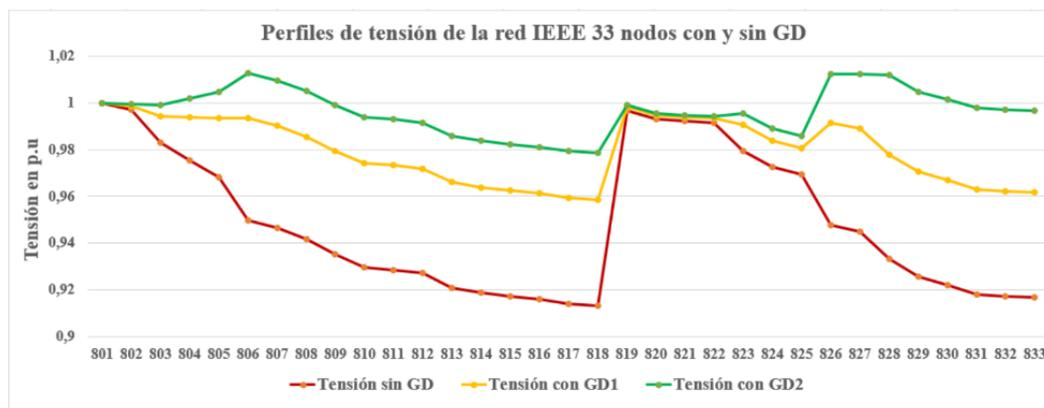
Figure 4. Voltage profiles in the 33-node IEEE system in three scenarios: without DG (red), with one DG (yellow) and two DG (green)
