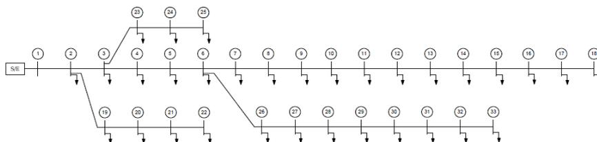
**Figure 1.** 33-node IEEE radial network topology.
