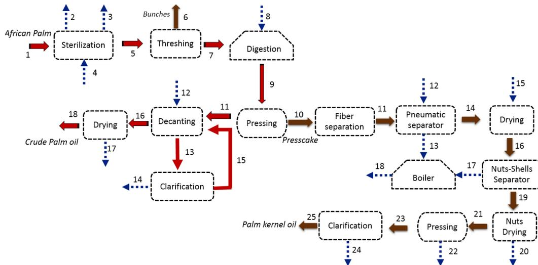
Figure 2. Block diagram for case 2
