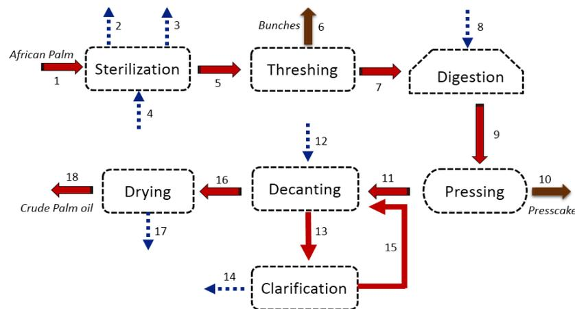
Figure 1: Block diagram for case 1
