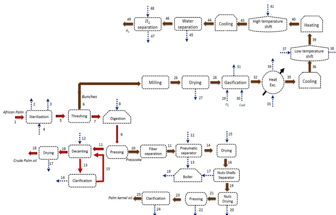
Figure 3. Block diagram for case 3
