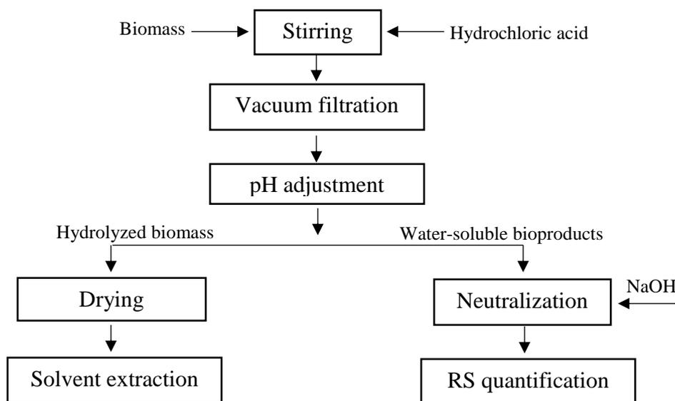
Figure 1. Experimental procedure for acid hydrolysis pretreatment.
