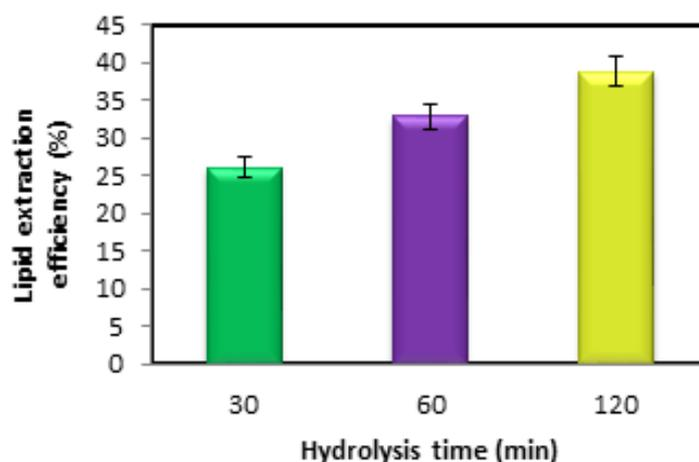
Figure 1. Effect of acid hydrolysis time on the increase of lipid efficiency for *Amphiprora* sp.
