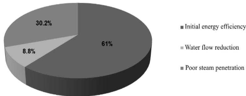
Figure 8. *Initial efficiency decrease in the condenser*
