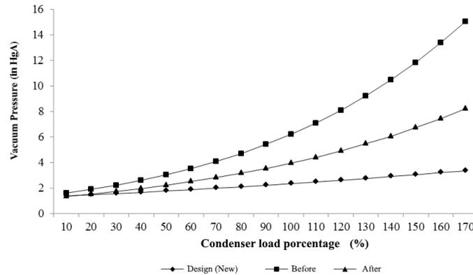
Figure 6. *Curves of condenser's performance.*
