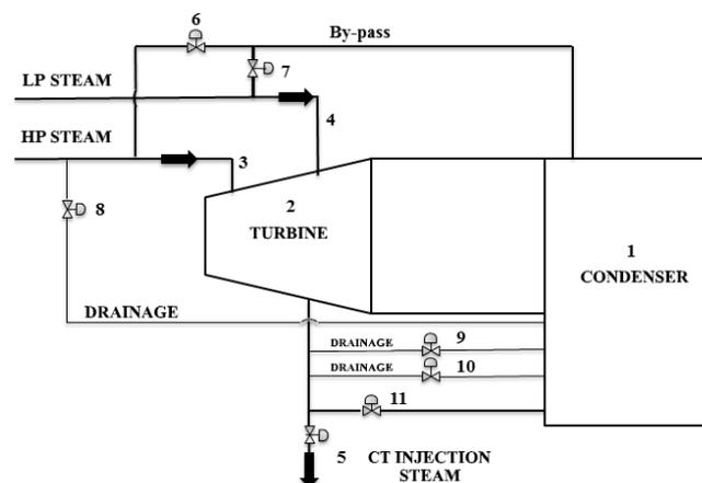
Figure 2. Scheme of steam-turbine system.
