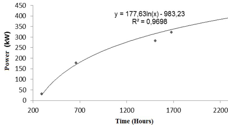
Figure 9. Performance degradation rate in the condenser
