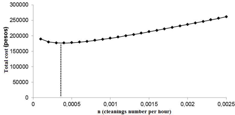
Figure 10. *Optimal cleaning frequency*
