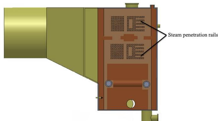
Figure 7. Actual configuration of the pipe bundles in the condenser
