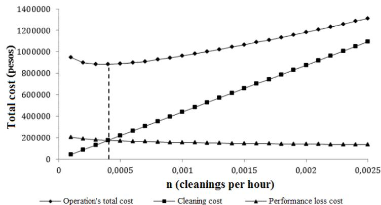
Figure 11. *Optimal cleaning frequency using the Hydrojet system*
