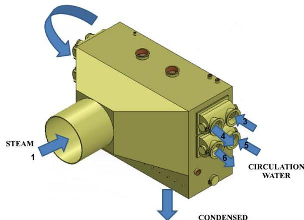
Figure 3. Schematic diagram of a surface condenser.
