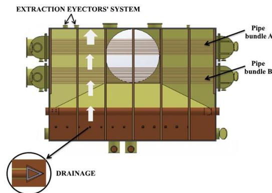
Figure 5. *Steam pass through condenser drains.*
