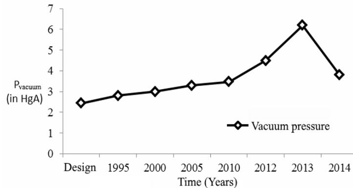
Figure 1. Increase of the vacuum pressure in the equipment
