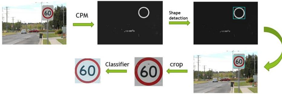
Figure 2: Flow Diagram of the traffic sign classification system
