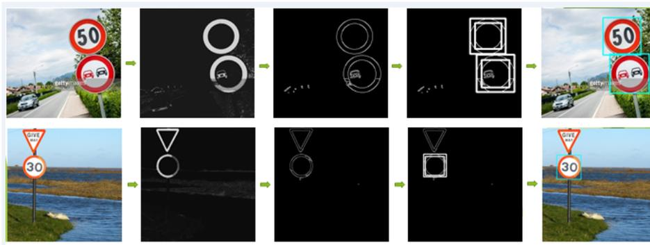
Figure 4: Examples of detection procedures
