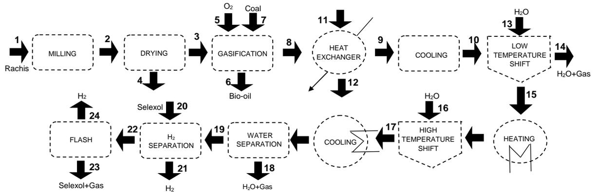
Figure 1. Process diagram of bio-hydrogen production process from palm rachis.
