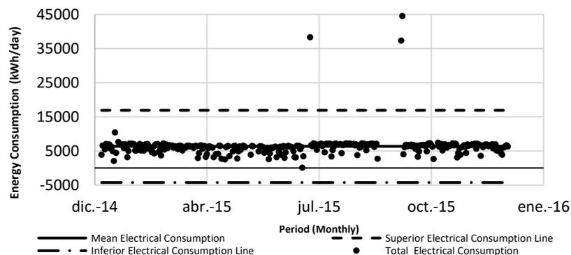
Figure 3. Control limit graph for the electric consumption of the pickling line.
