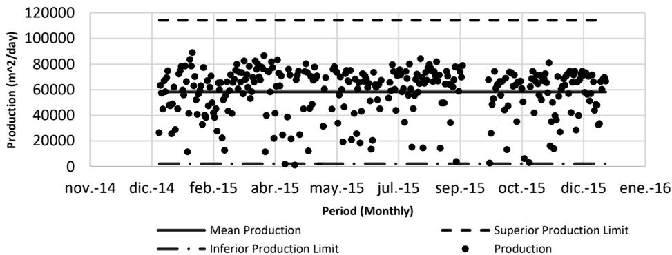
Figure 4. Control limit graphic for the production of the pickling line.
