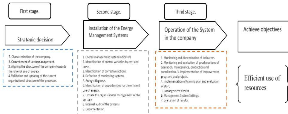
Figure 1. Components in energy management system
