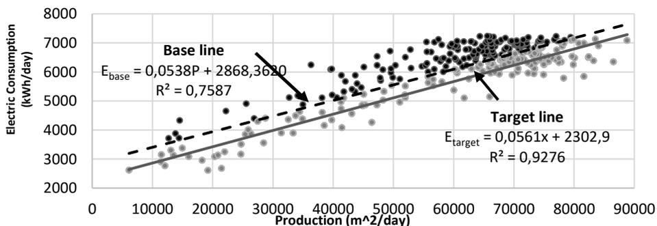
Figure 5. Target line graph for pickling line.
