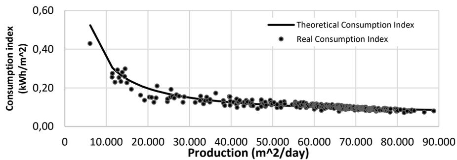
Figure 6. Actual consumption index vs. theoretical consumption index for the pickling line.
