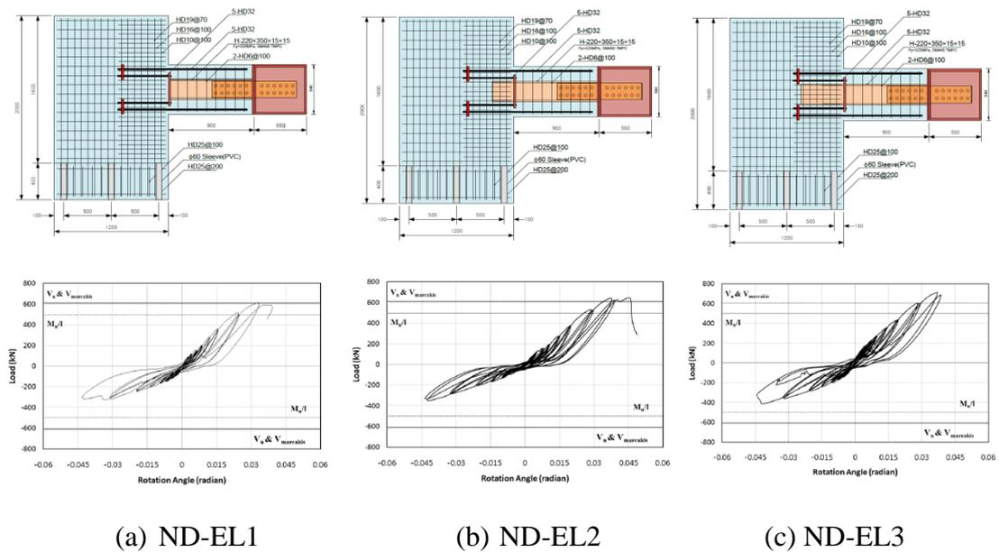
Figure 2. Effect of embedment length on the behavior of SRC coupling beam [4]
