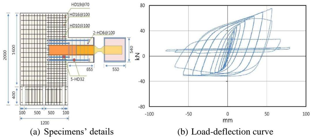
Figure 4. Response of SRC coupling beam with steel damper [6]
