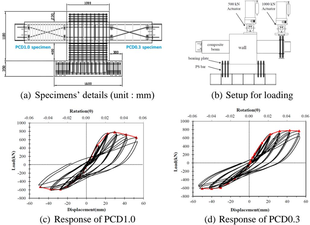
Figure 3. Effect of stirrup on the behavior of prestressed SRC coupling beam [5]
