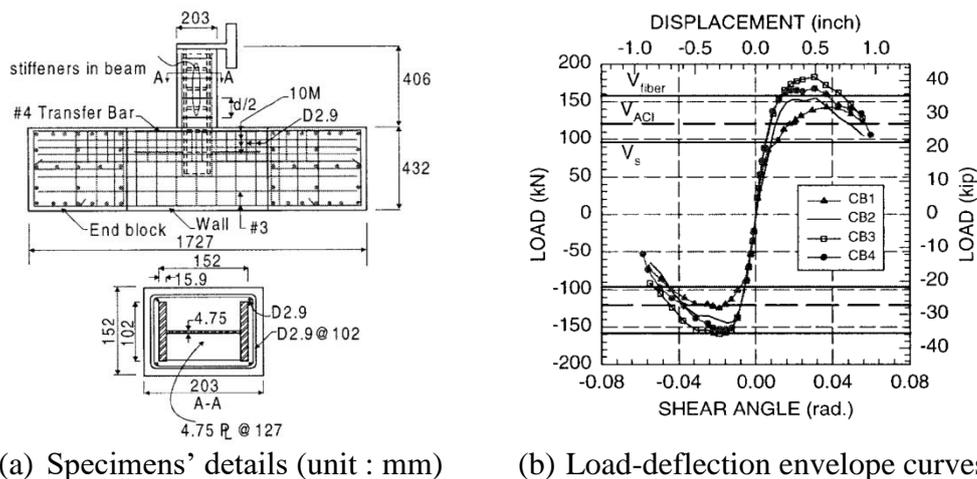
(a) Specimens' details (unit : mm) (b) Load-deflection envelope curves
