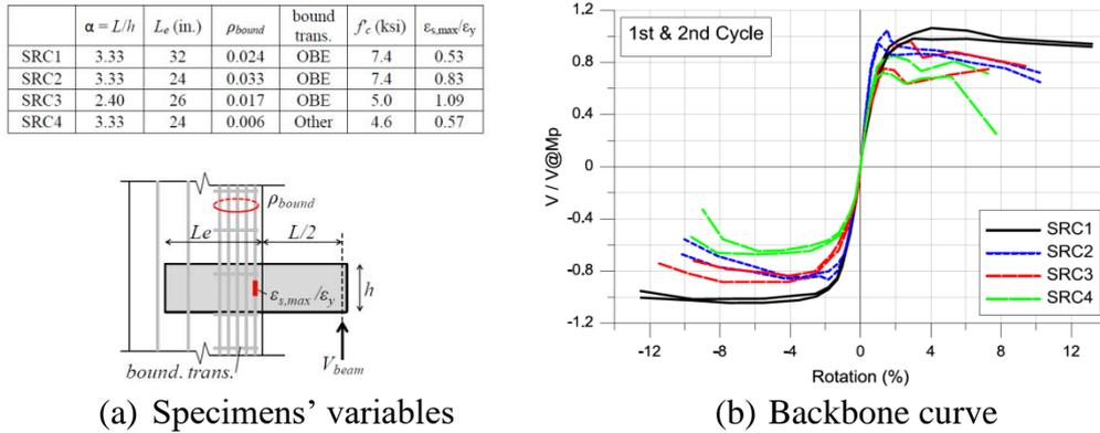
Figure 5. Response of SRC coupling beam [7]
