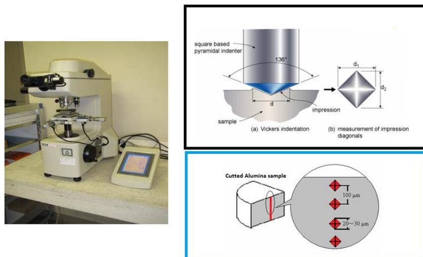
Fig. 1 Experiment for Vickers hardness
