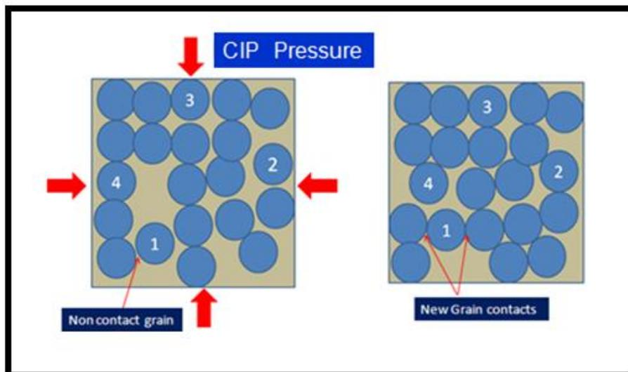
Fig. 4 Effect of CIP on grains contact
