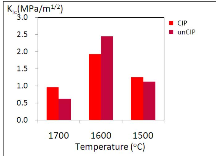
Fig. 3 Fracture Toughness of microwave sintered alumina for CIP and unCIP samples
