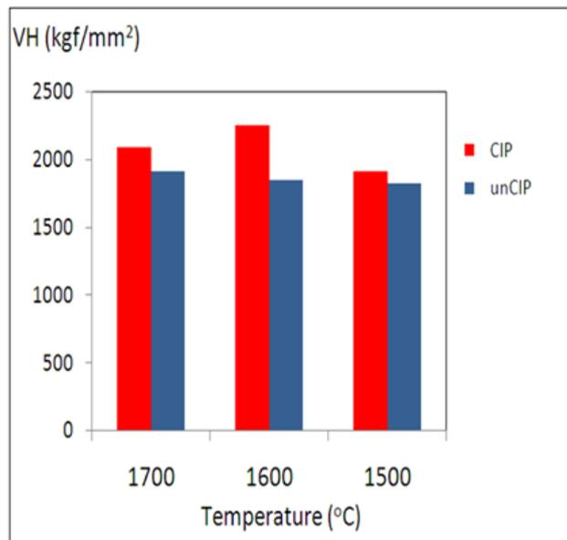
Fig. 2 Micro Vickers hardness of microwave sintered alumina
