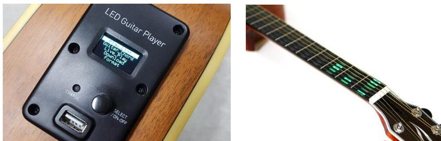
Figure 4. A prototype of GuitarSolo; A controller (left) and LED fretboard (right)
