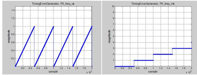
Figure 3:  $u_k$  and  $m_k$  Output of the Timing Error Generator in +ppm.
