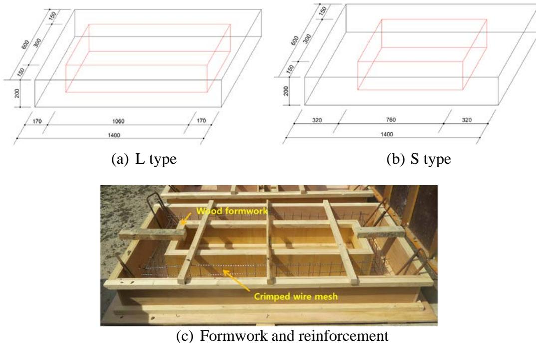
Fig. 1 Configuration and dimension of concrete cask storage (unit : mm)
