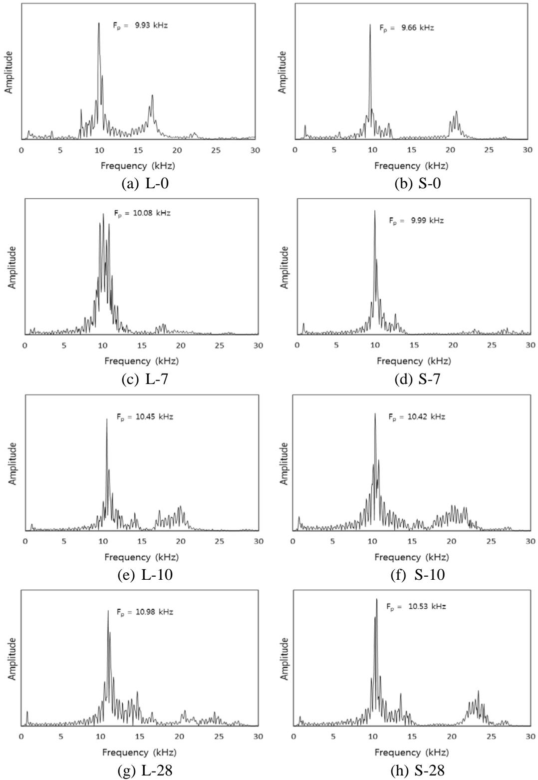
Fig. 4 Typical amplitude spectrum of concrete casks from impact-echo tests
