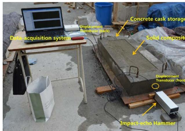
Fig. 2 System for measuring impact-echo response of concrete cask storage
