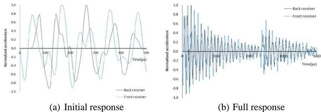
Fig. 3 Typical acceleration waveforms of L type concrete cask storage
