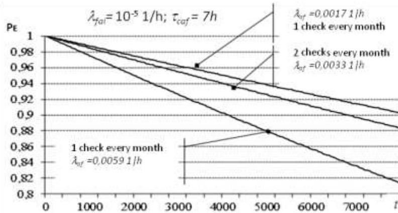
Fig.3. Change of efficiency of use CTS in case of autonomous functioning
