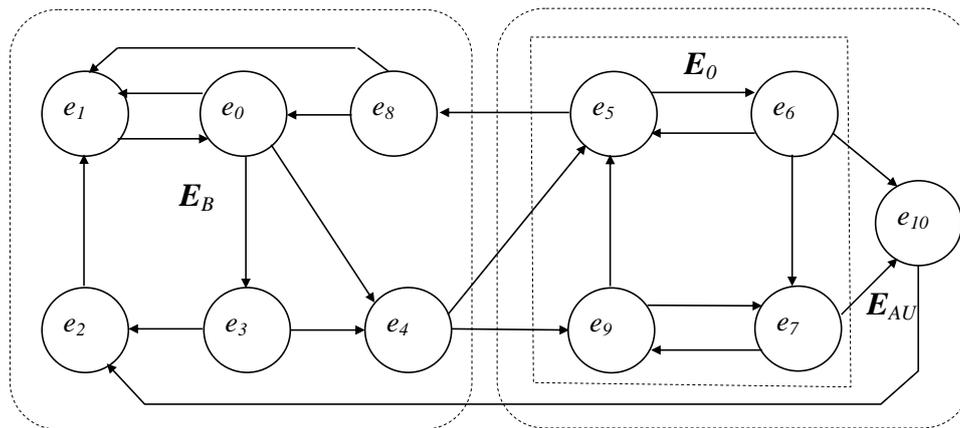
Fig.1 Graph of model's statuses and transitions when CTS in the process of operation
