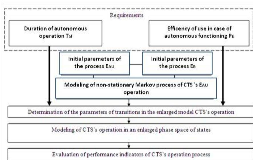
Fig.4 The general scheme of modeling of CTS's operation process
