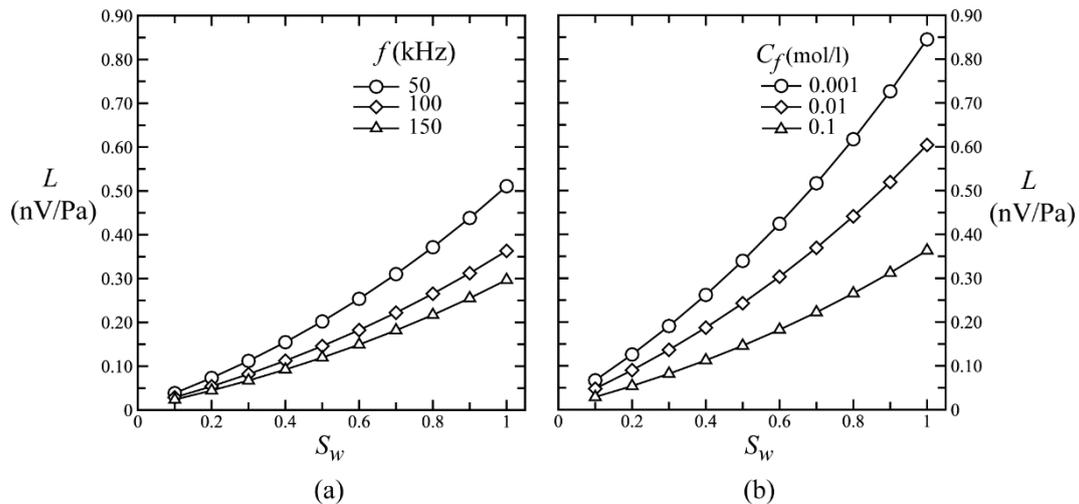
**Fig. 3** Effect of water saturation on coupling coefficient. (a)  $C_f = 0.1$  mol/l, (b)  $f = 100$  kHz.
