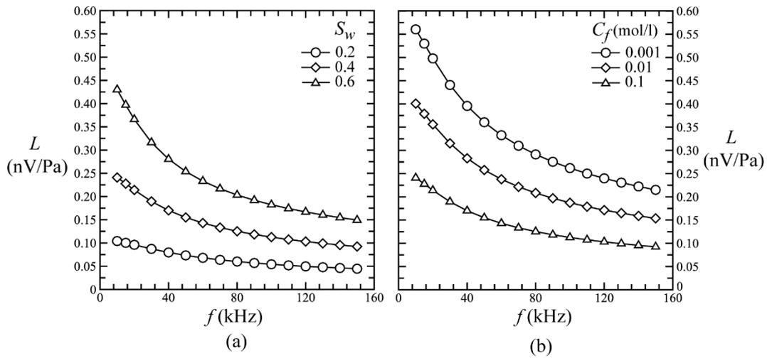
**Fig. 4** Effect of frequency on coupling coefficient. (a)  $C_f = 0.1$  mol/l, (b)  $S_w = 0.4$
