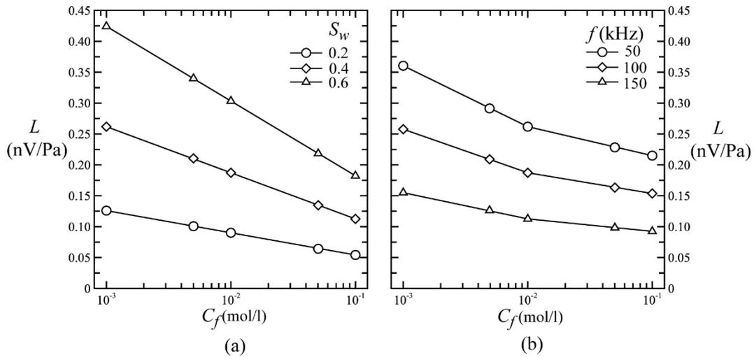
**Fig. 2** Effect of brine concentration on coupling coefficient. (a)  $f = 100$  kHz, (b)  $S_w = 0.4$
