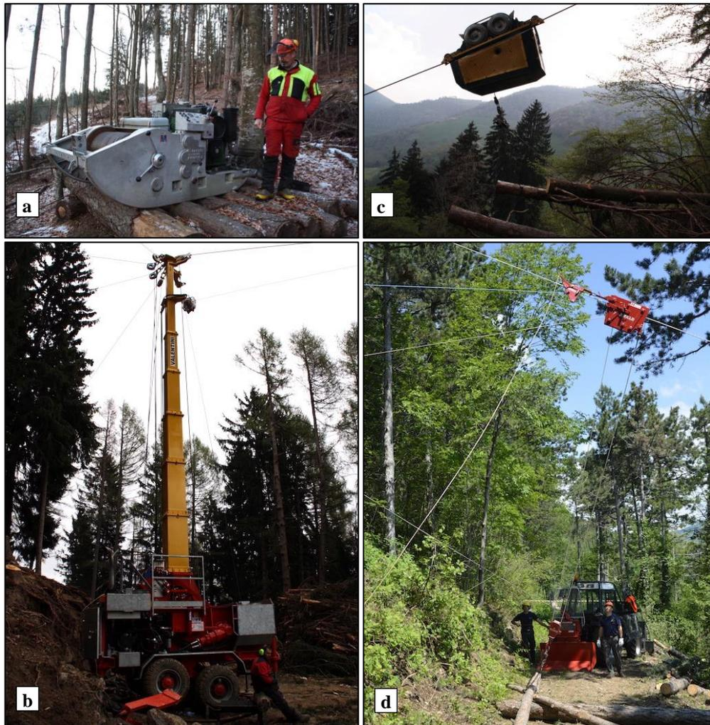
Fig. 2: a) Sled yarder; b) Mobile tower yarder; c) Self-propelled carriage-based yarder; d) Mobile yarder without a tower
