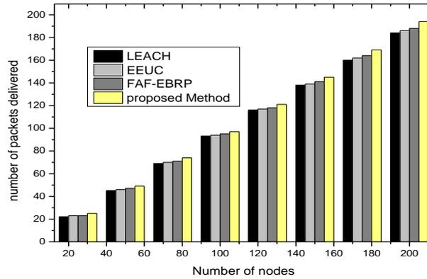
Figure 5: Estimation of packet delivery in proposed protocol with LEACH, EEUC and FAF-EBRP
