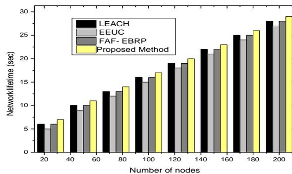
Figure 4: comparison of network lifetime in proposed protocol with LEACH, EEUC and FAF-EBRP
