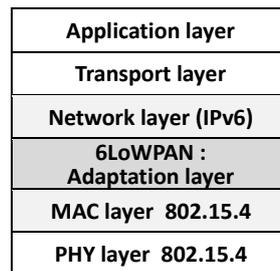
**Figure 2.** The position of 6LoWPAN in the protocol stack.
