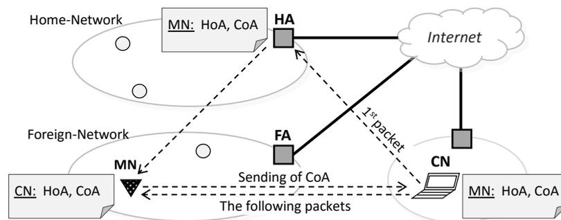
**Figure 5.** A communication scenario between a CN and a MN using MIPv6.
