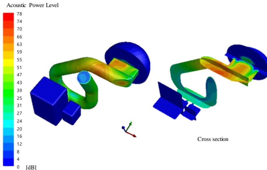
Fig 5. Acoustic power level at 5000rpm
