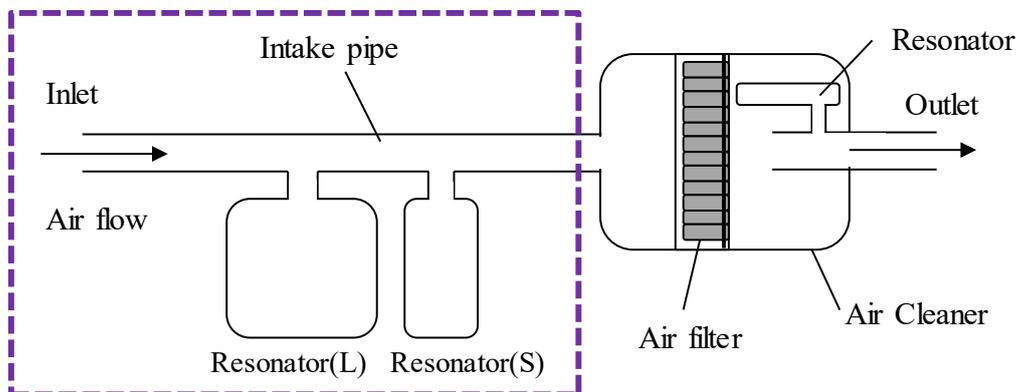
Fig 1. Schematic diagram of air intake system
