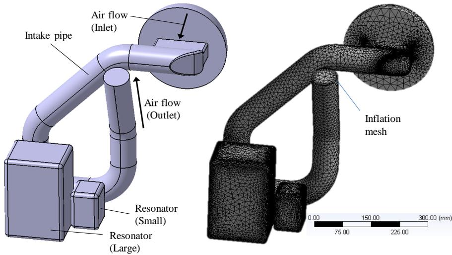
Fig 2. Air intake system model and meshes
