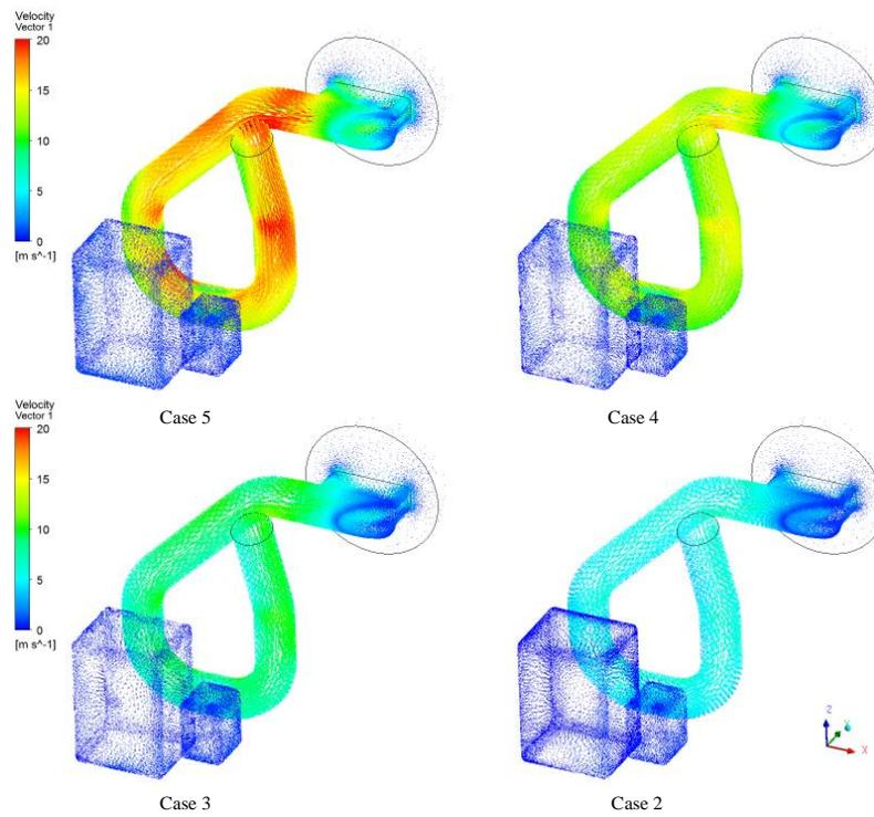
Fig 3. Velocity flow of intake system
