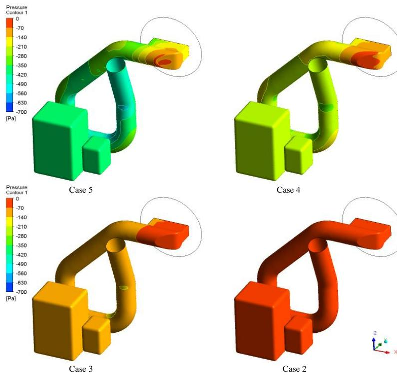
Fig 4. Pressure of intake system
