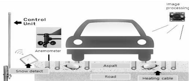
Fig1. IoT based snow melting system composition
