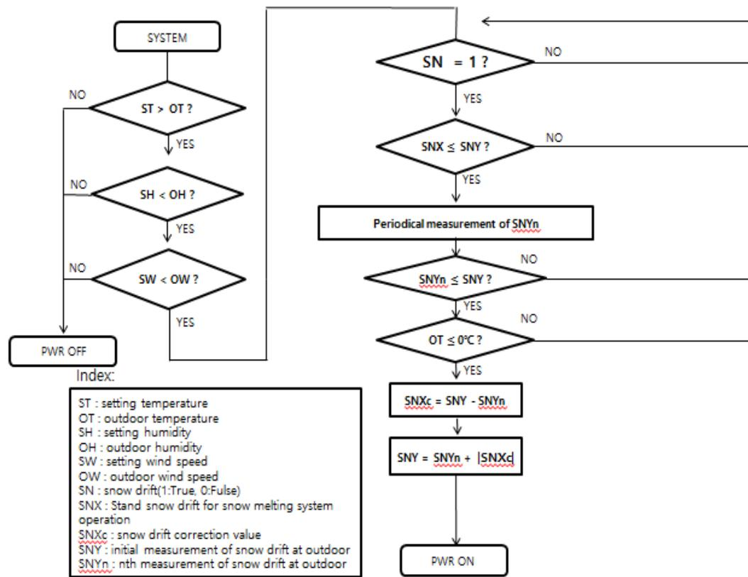
Fig4. snow melting system operation algorithm considering the alteration of snow drift
