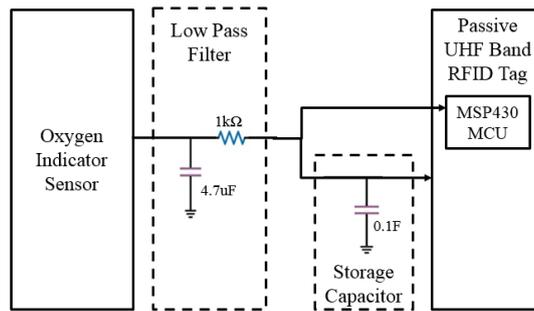
Fig.6. Interface circuit
