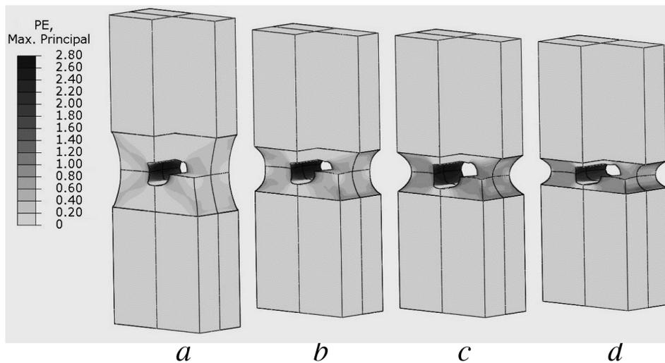
Figure 4: The total deformation distribution in the simulated specimens with various thickness values of Al interlayer at the moment of initial FEM cell rupture: 1 — 5 mm; 2 — 2.5 mm; 3 — 1.8 mm; 4 — 1.25 mm
