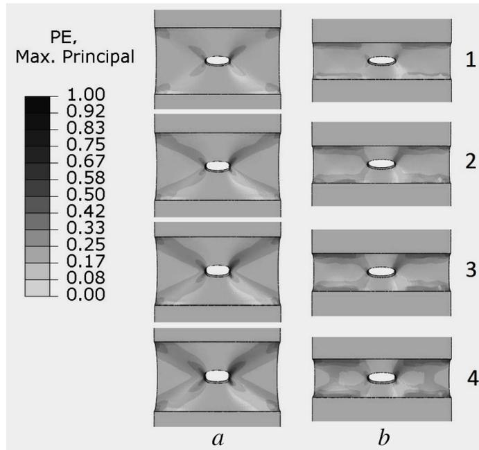
Figure 1: Distribution of the plastic deformation in Al interlayer with the thickness value of (a) 5 mm; (b) 1.25 mm at the relative interlayer deformation value of: I –  $\epsilon = 5\%$ ; II –  $\epsilon = 6.5\%$ ; III –  $\epsilon = 7.8\%$ ; IV –  $\epsilon = 10\%$
