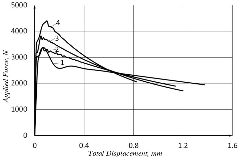
Figure 2: Absolute axial deformation of the specimen - applied force curves for the simulated interlayer thickness values: 1 — 5 mm; 2 – 2.5 mm; 3 – 1.8 mm; 4 – 1.25 mm
