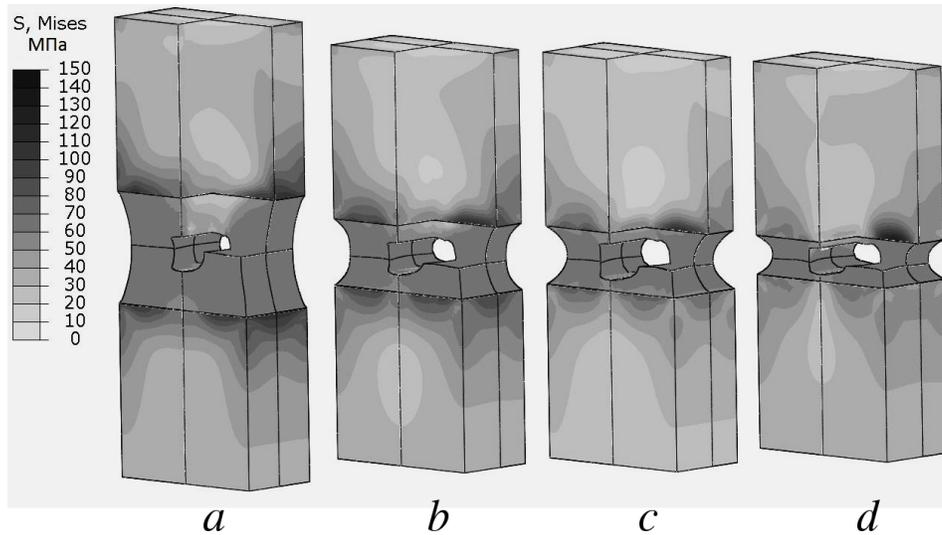
Figure 3: Von Mises stress distribution in the simulated specimens with various thickness values of Al interlayer at the moment of initial FEM cell rupture: 1 — 5 mm; 2 — 2.5 mm; 3 — 1.8 mm; 4 — 1.25 mm
