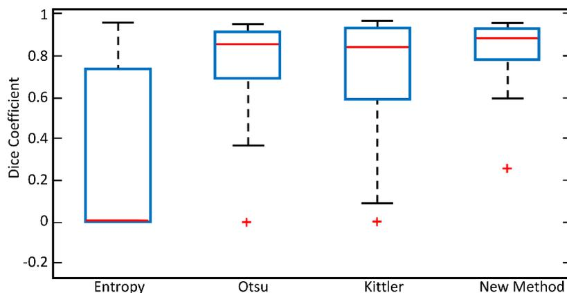
**Figure 4.** Box plot of Dice coefficients of the method with different criterion functions for threshold localization
