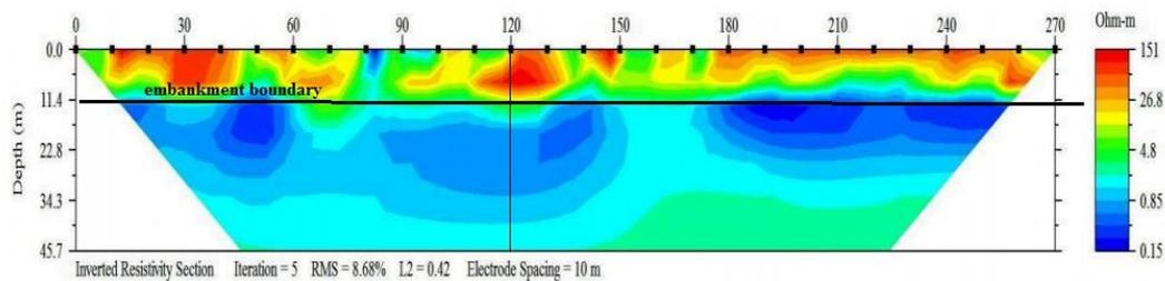
Fig.4 2D Resistivity imaging in P.79 – P.82 LUSI (Lumpur Sidoarjo) embankment [10]
