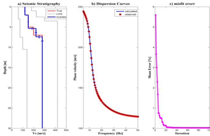
Fig.1 Inversion result of noise-free data. (a) Seismic stratigraphy or  $V_s$  profile; (b) Fitting between observed data and calculated data; (c) misfit error as an iteration function
