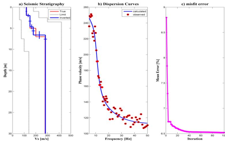
Fig.2 Inversion result of noise-contaminated data. (a) Seismic stratigraphy or  $V_s$  profile; (b) Fitting between observed data and calculated data; (c) misfit error as an iteration function
