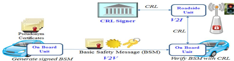
Fig.2 Certificate Verification Process
