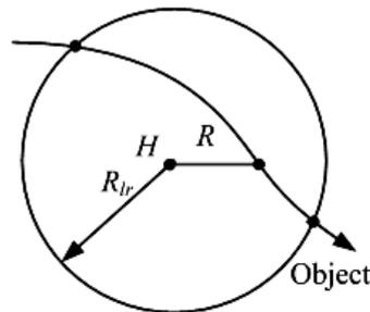
Figure 3. Object trajectory in the area of SRWD action
