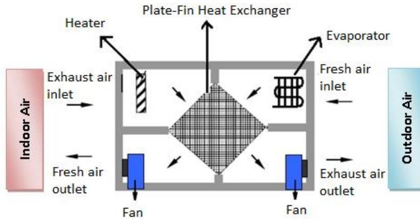
Fig. 2 Schematic representation of the testing apparatus
