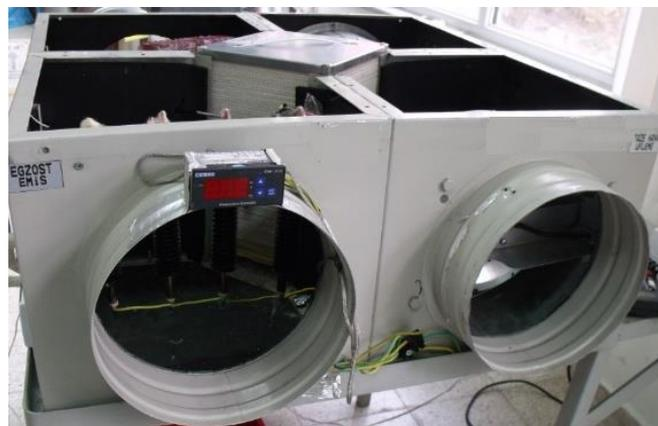
Fig. 3 The heat recovery device used in the test
