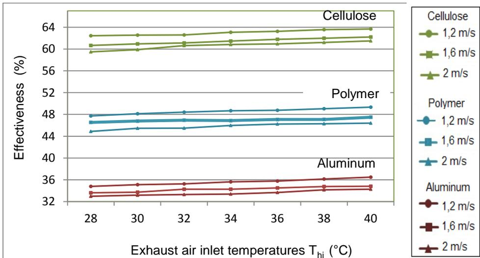
Fig. 7 Comparison of effectiveness of the aluminum, polymer and cellulose heat exchangers where the fresh air inlet temperature is 10 °C
