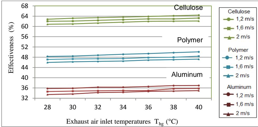
Fig. 6 Comparison of effectiveness of the aluminum, polymer and cellulose heat exchangers where the fresh air inlet temperature is 0 °C at different air rates
