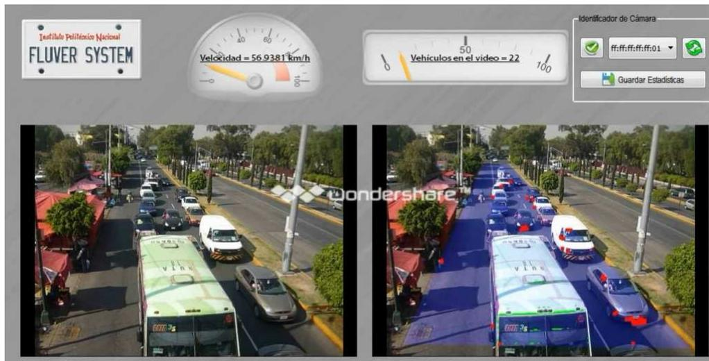
Fig. 8: System that detects the average speed and traffic flow.
