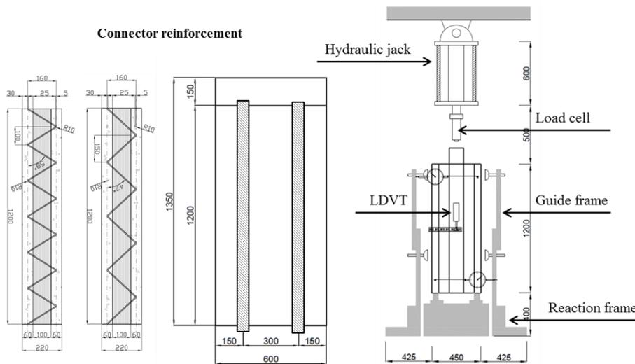
**Figure 1** Reinforcement details of specimen and test set-up
