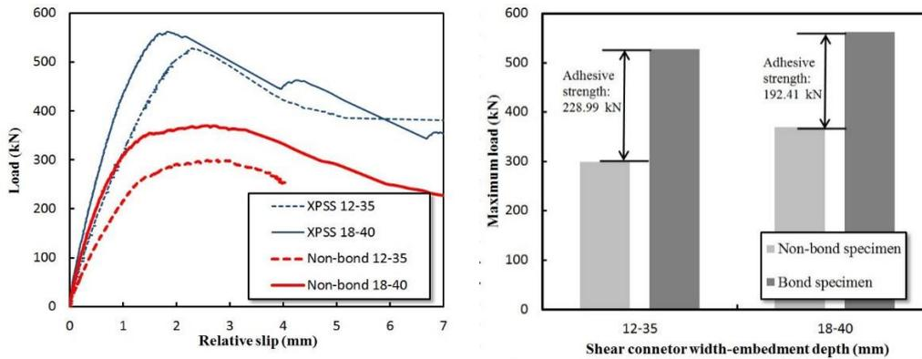
(a) In-plane shear behavior of specimens
