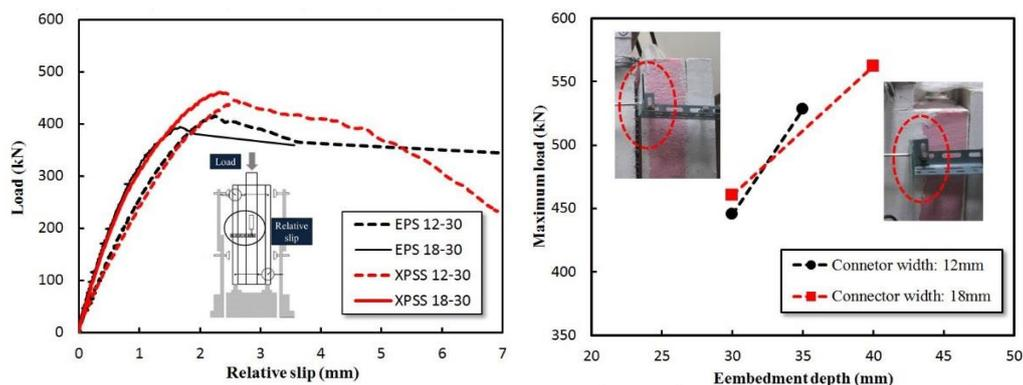
(a) Effects of insulation and shear connector pitch
