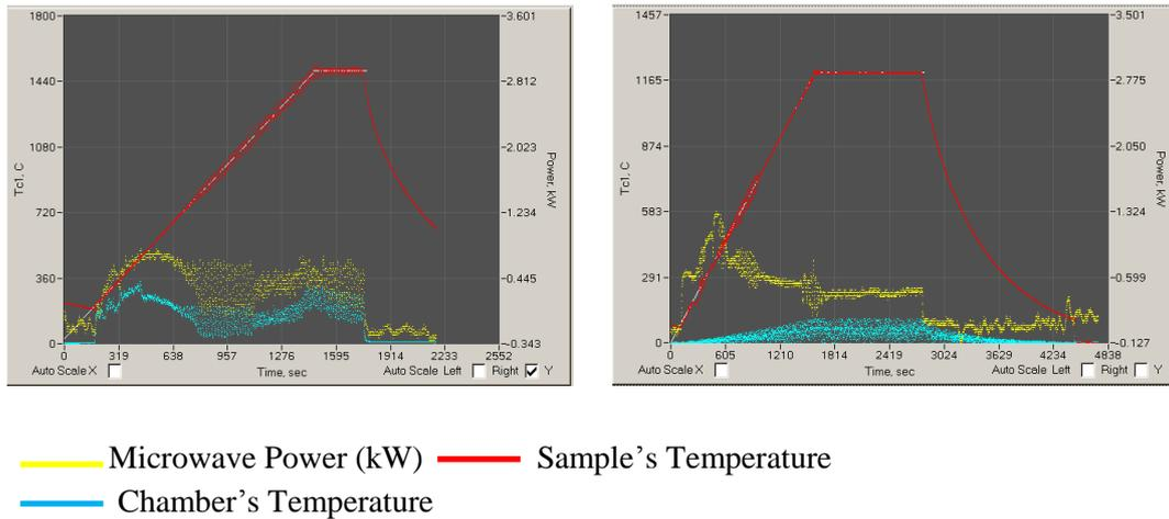
Figure 1. Temperature profile as function of time of MMW sintering of silica and alumina ceramics
