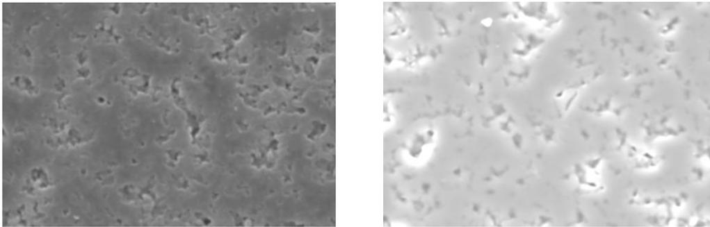
Figure 4. SEM photos of porosity of alumina ceramics sintered at 1400°C by (1) MMW (left) and (2) conventional sintering (right)
