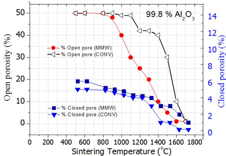
Fig. 3 Reduction of open and closed porosity of alumina upon MMW as compared to conventional sintering
