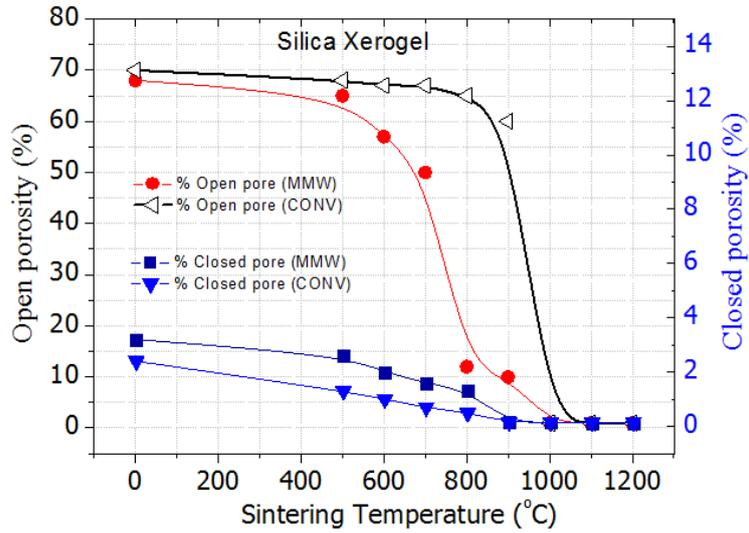
Fig. 2 Reduction of open and closed porosity of silica xerogel upon MMW as compared to conventional sintering
