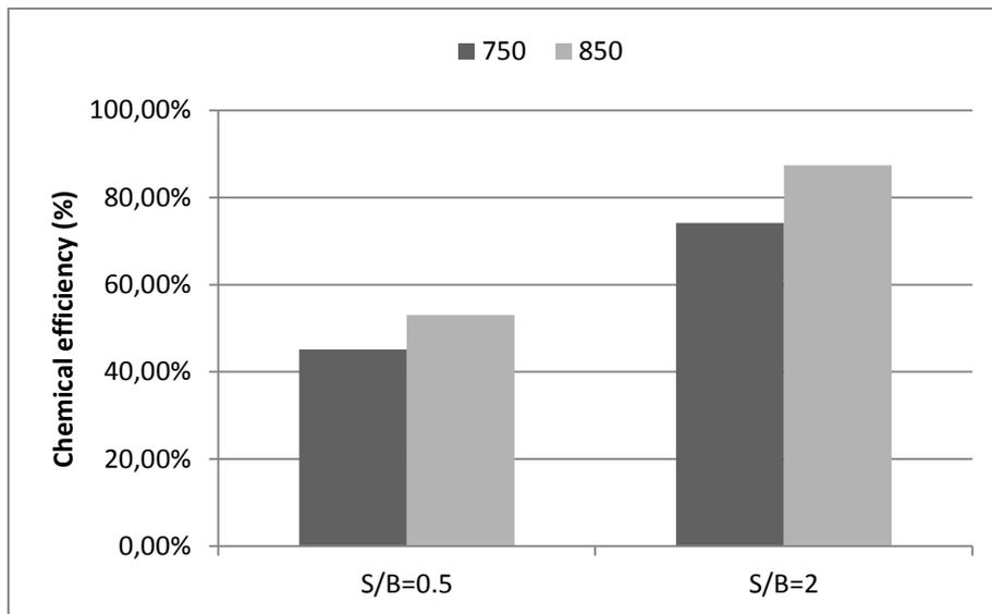
Figure 1 Hydrogen chemical efficiency at the output of the catalytic filter candle
