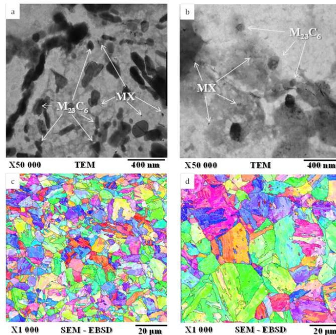
Fig.3 Microstructure and orientation maps of 9Cr-3Co-2W-MoVNb steel with 0,1wt.% (a, c) and 0.014wt.%(b,d) of carbon
