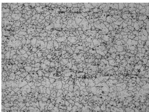
Fig.5 – Microstructure of 15Cr-16Ni-2Mo-Ti-B steel (x200)
