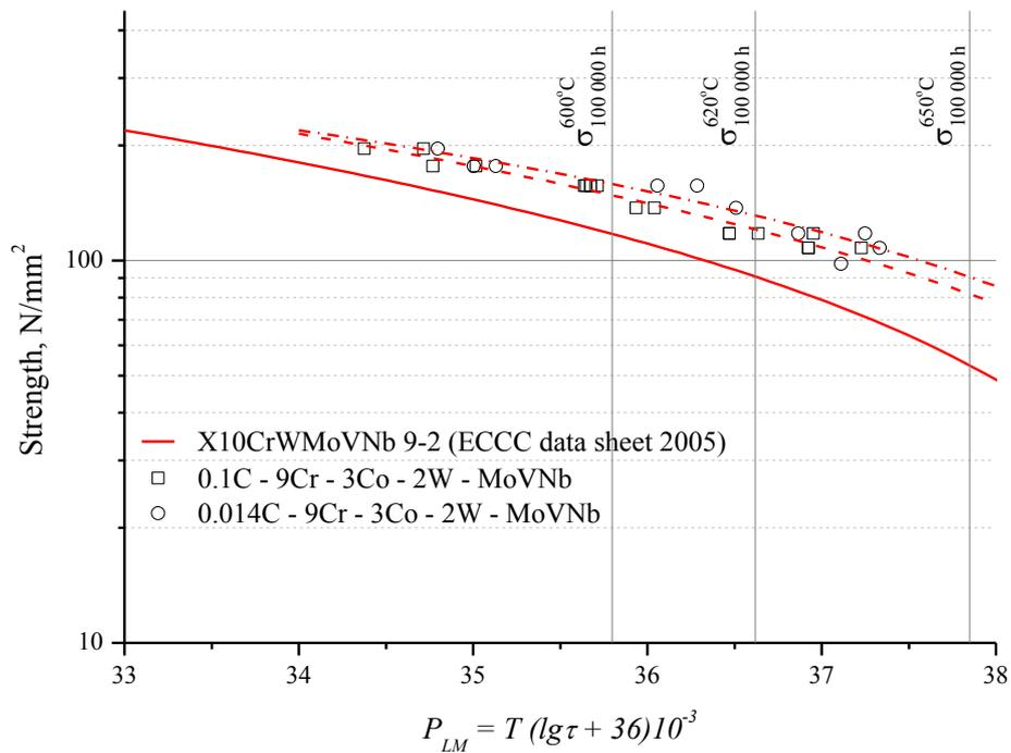
Fig.4 Creep data of tempered P92 steel and 9Cr-3Co-2W-MoVNb steel
