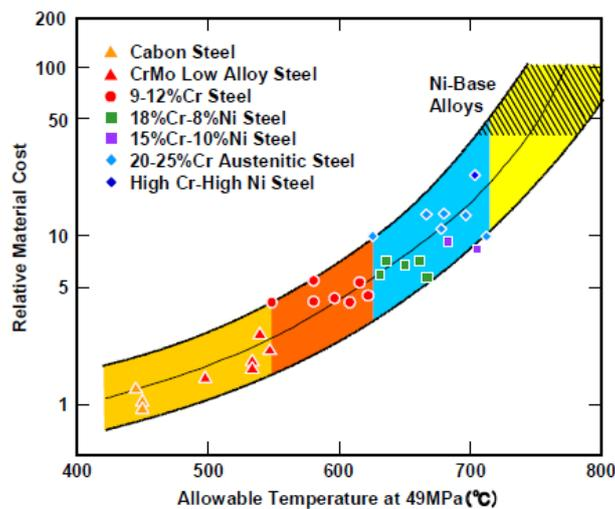
Fig.1 - Comparison of relative material cost with allowable temperature at 49MPa [1]
