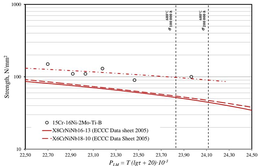
Fig.6 - Creep data of 15Cr-16Ni-2Mo-Ti-B, X8CrNiNb16-13 and X6CrNiNb18-10 steels
