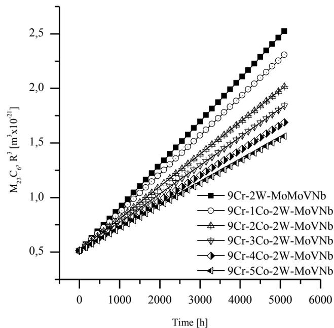
Fig.2 Time dependent coarsening of  $M_{23}C_6$  at  $650^\circ\text{C}$  in  $9\text{Cr-}x\text{Co-}2\text{W-MoVNb}$  ( $x = 0 - 5$  wt.%)
