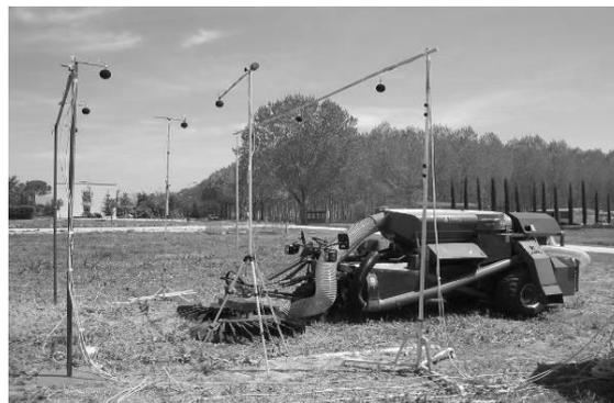
Fig. 8 - The tested machine with 8 microphones at a 3 meter height
