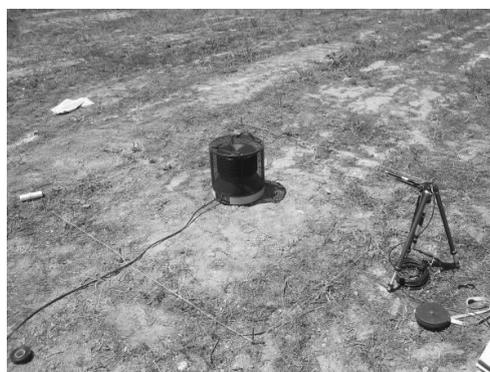
Fig. 9 - Tested point source and microphone placed on apposite pole
