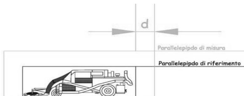
Fig. 6 - Scheme of the “ $d$ ” distance between the measurement and the set parallelepiped
