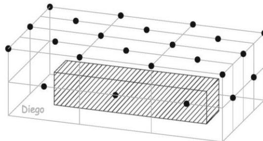
Fig. 7 - Scheme of the microphone locations: the internal parallelepiped contains the machine, while on the external one the microphone positions are highlighted
