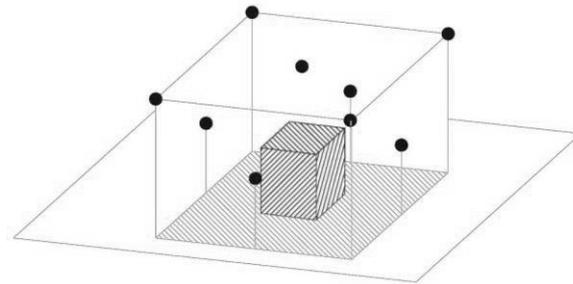
Fig. 10 - Scheme of the Bruel & Kjaer “4204” source (in the middle) and the microphone locations around it
