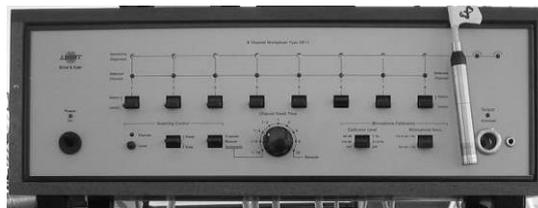
Fig. 2 - Bruel & Kjaer “2711” model multiplexer with 8 channels
