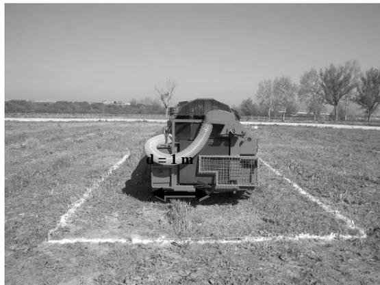
Fig. 5 - Facma Cimina 300 S machine placed in the centre of the measurement parallelepiped
