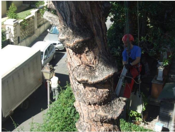
Figure 1- Tree climber with Resistograph analyzing wood resistance
