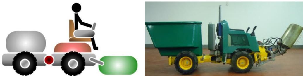
Figure 1 – (left) Scheme of the studied articulated tractor; (right) overview of one of the first prototypes equipped with a front-coupled mower and a rear dumper
