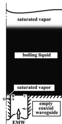
Fig. 1. The simulation area and initial distribution of liquid and vapor phases of n-heptane. A piece of border ABC is permeable to microwaves and impermeable to n-heptane. The input of the microwave power is marked by the arrow
