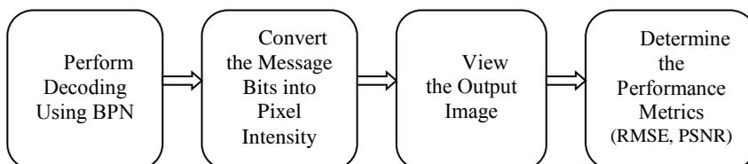
**Fig.2.** Decoding at the receiver end
