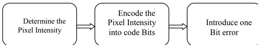
**Fig.1.**Encoding at the transmitter end
