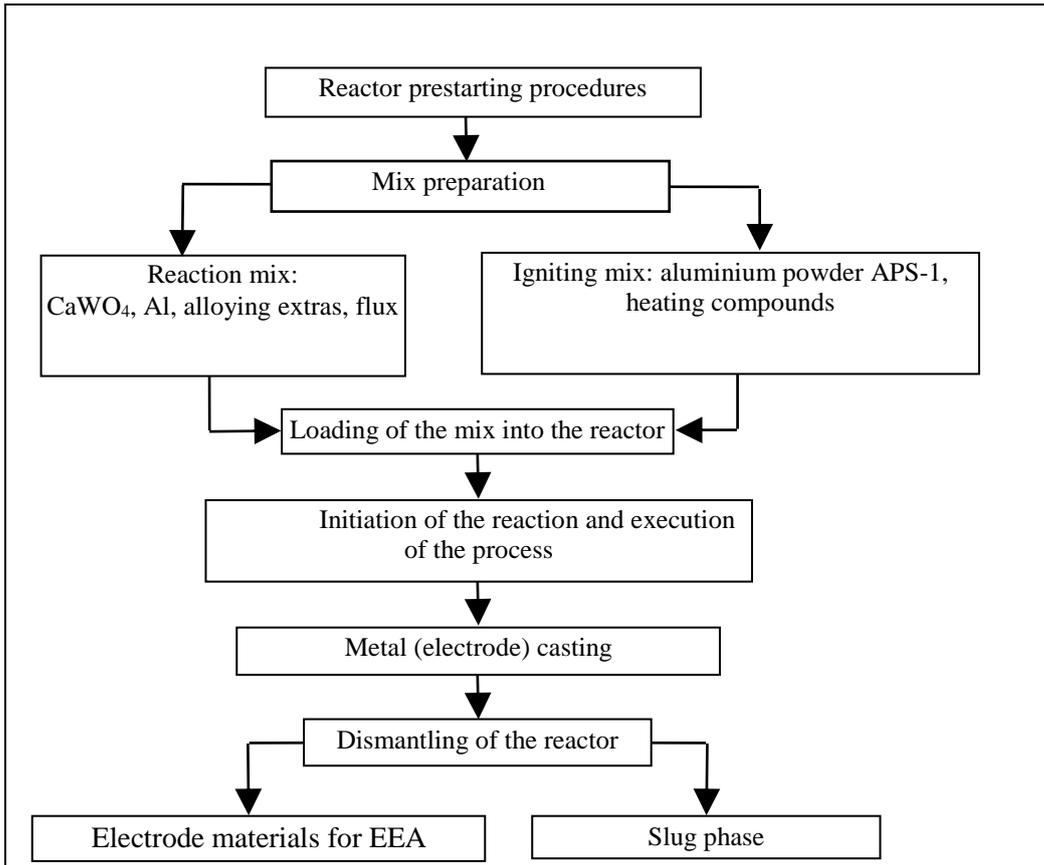
Fig. 1. Technological scheme of the producing of electrode materials
