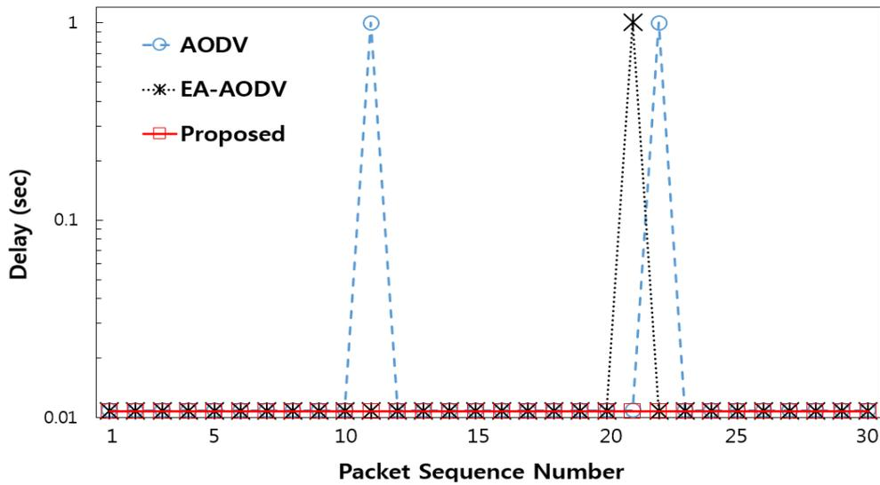
Figure 3. End-to-end delay of packet in 3x3 topology
