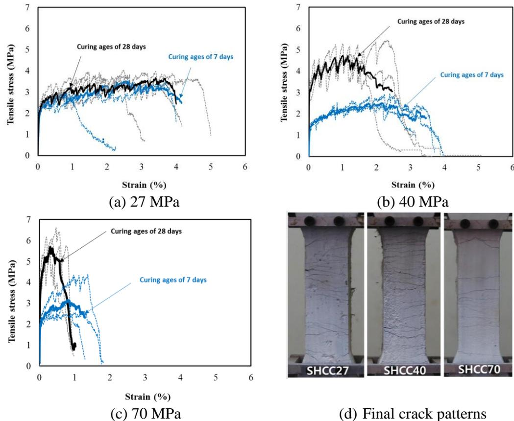
Figure 2. Tensile and cracking behaviors of sustainable SHCCs
