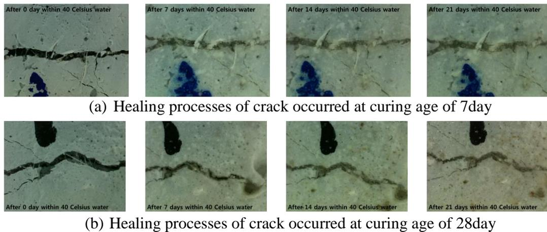
Figure 3. Typical crack-healing behavior of SHCC27 in 40 Celsius water
