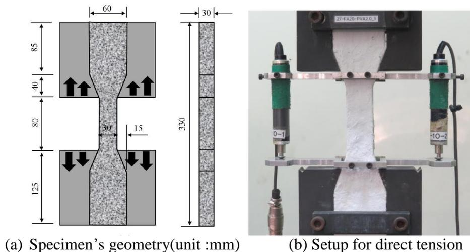
Fig. 1. Specimen configuration and setup for direct tension tests
