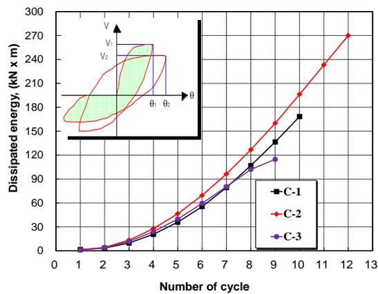
Fig. 6 Dissipated energy
