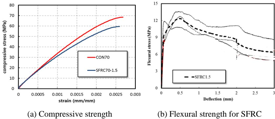
Fig. 2 Mechanical properties
