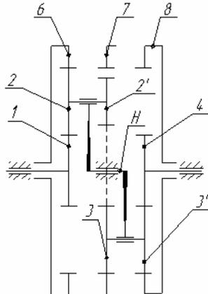
Figure 2: Kinematic diagram of the eight-speed planetary gearbox
