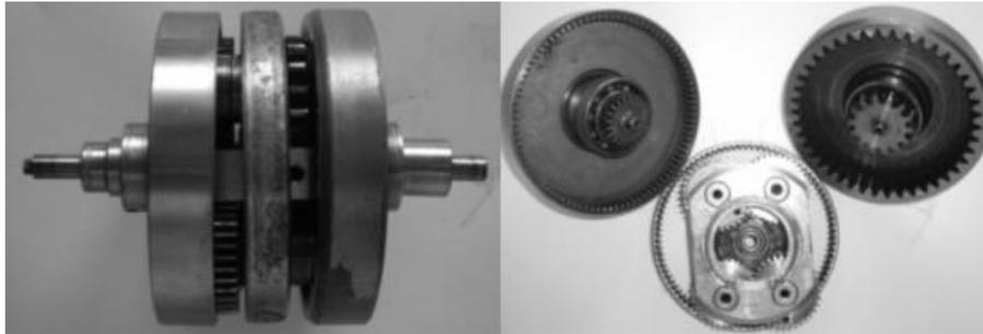
Figure 1: The design of the planetary system of universal multi-threaded differential mechanism
