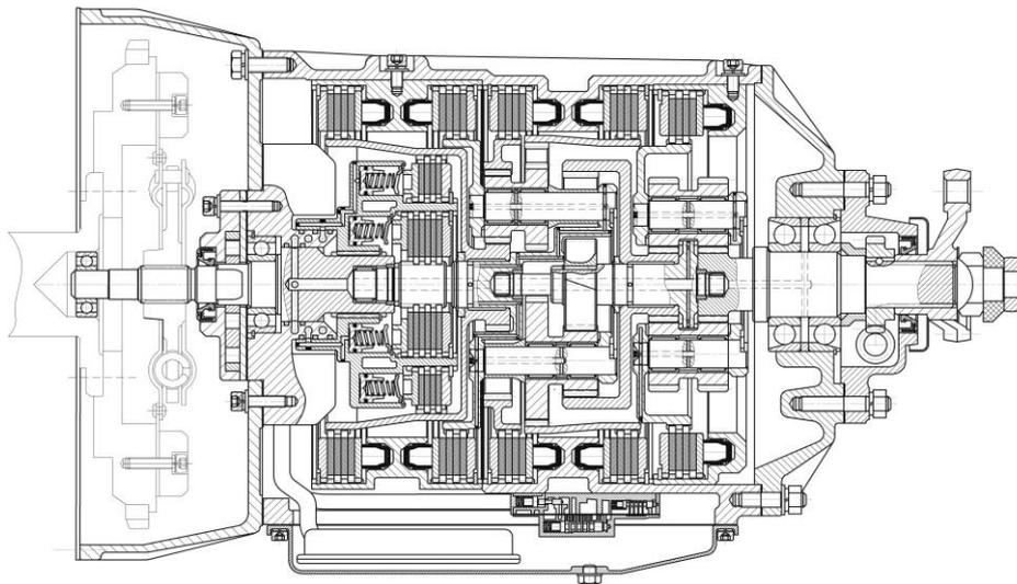
Figure 3: The design of the eight-speed planetary gearbox on the basis of universal multi-threaded differential mechanism
