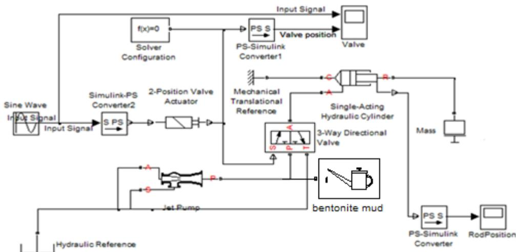
Fig. 2 Numerical model of mud circuit ((SIMHYDRAULICS))
