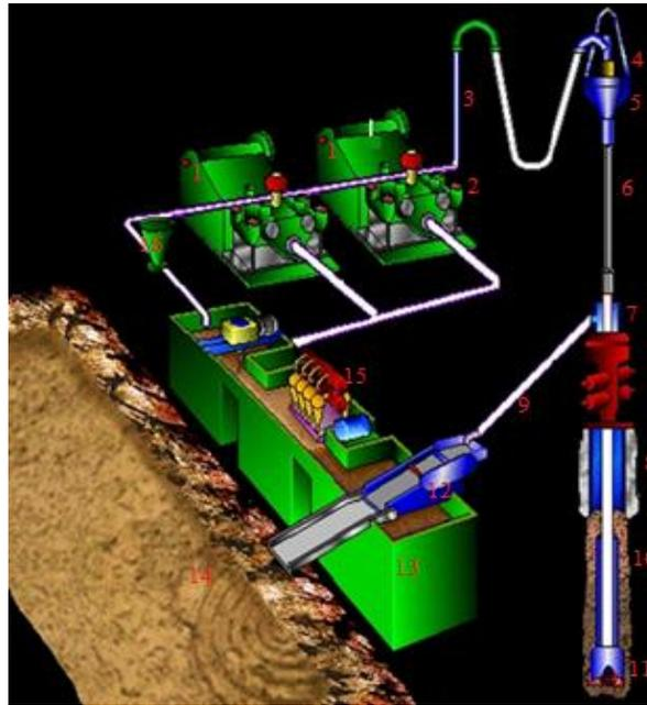
Fig. 1 Drilling mud circuit
