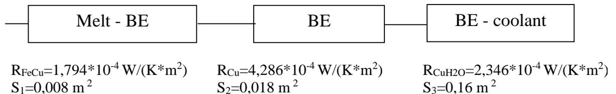
Figure 3: Thermal resistances attributed to  $1 \text{ m}^2$ .
