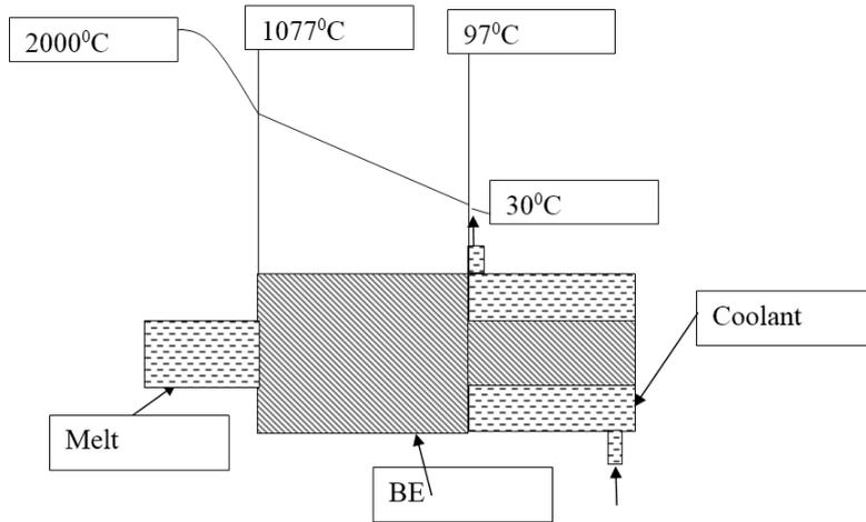
Figure 4: System "melt - BE - coolant (water)."
