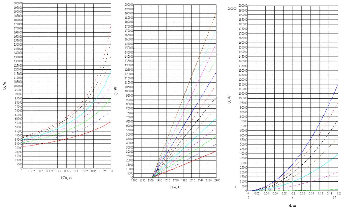
Figure 5: Graphs of the critical heat flow as a function of the diameter of contact with the molten BE, BE length and temperature of the melt.
