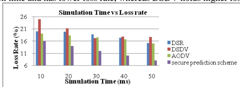
Figure 8: Analysis of Simulation time vs loss rate for AODV, DSR, DSDV and secure prediction scheme
