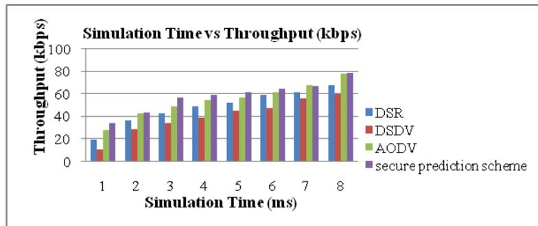
Figure 6: Analysis of Simulation time vs Throughput for AODV, DSR, DSDV and secure prediction scheme
