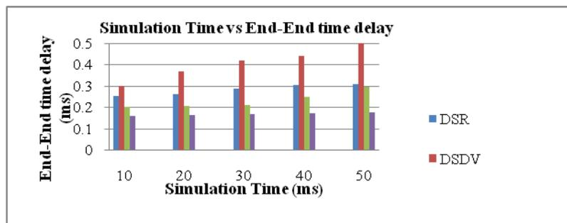
Figure 7: Analysis of Simulation time vs End-End time delay for AODV, DSR, DSDV and secure prediction scheme
