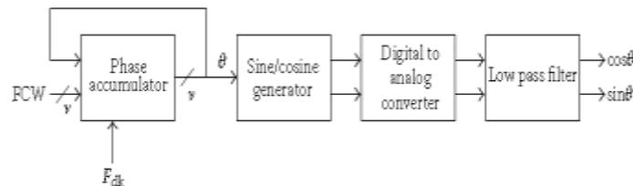
**Figure 1: Simplified Block Diagram of DDFS**
