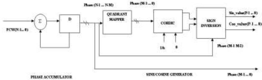
Figure 4: Block Diagram of CORDIC based DDFS
