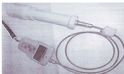
**Fig. 3: Smart SG-1R Probe connected to RADIAGEM 2000**
