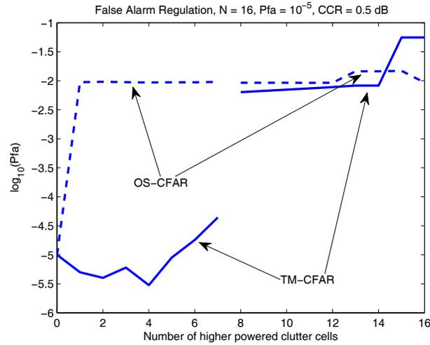
Figure 20: Clutter transitions in vertically polarised clutter, with a 0.5 dB clutter power increase.
