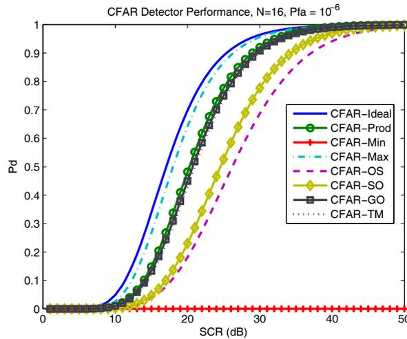
Figure 6: Detector performance in homogeneous vertically polarised clutter.
