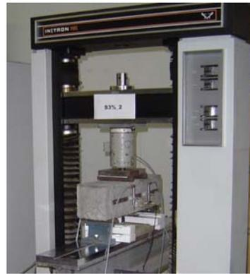
Fig. 2. Bending test setup.
