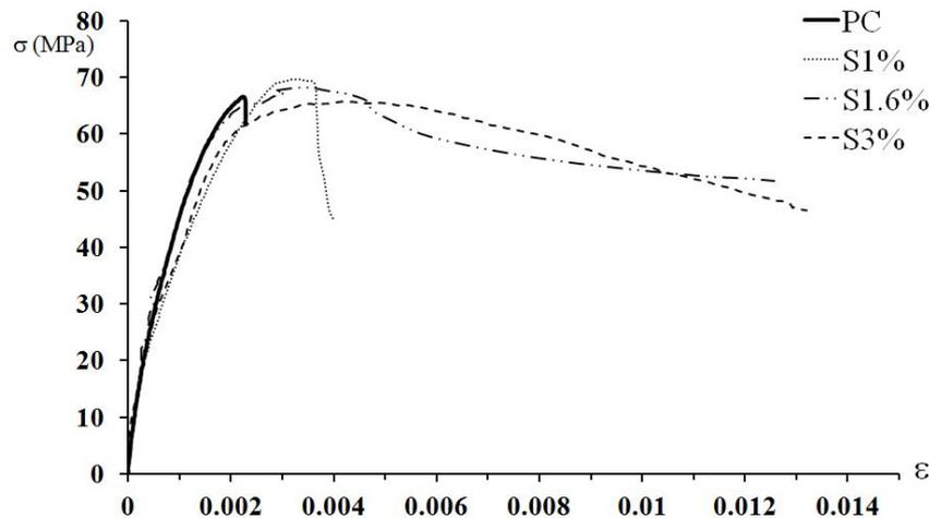
Fig. 3. Typical stress-strain compression curves.
