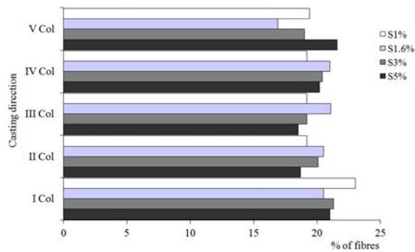
Fig. 6. Comparison of fibre dispersion on fracture surface.
