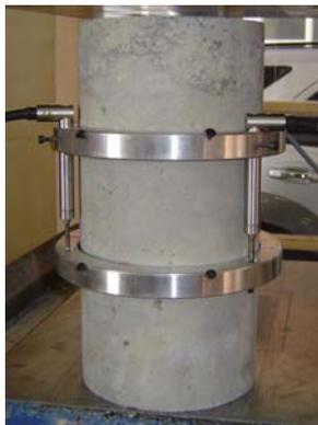
Fig. 1. Compressive test setup.
