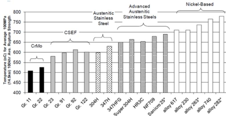
Fig. 3: Heat strength properties of various steels
