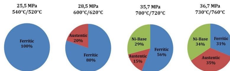
Fig. 2: Different steel properties necessary depending on steam turbine unit parameters
