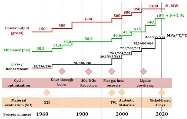
Fig. 1: The evolution of steam turbine unit operating parameters
