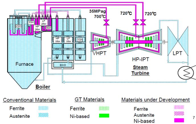
Fig. 5: Choice of steels for A-USC steam-turbine generator units
