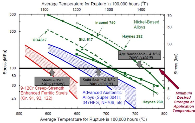
Fig. 4: Application ranges for various steels
